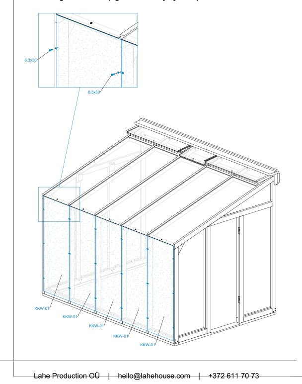
NB! Do not over tighten screws (tighten carefully by hand)!
