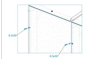
Placing glass to correct position on frame will be done on site by installer. For a best result it is important to check that glass is correctly positioned, gaps are equal and screws line up. We recommend using laser leveling tool or similar device for aligning screwheads.
