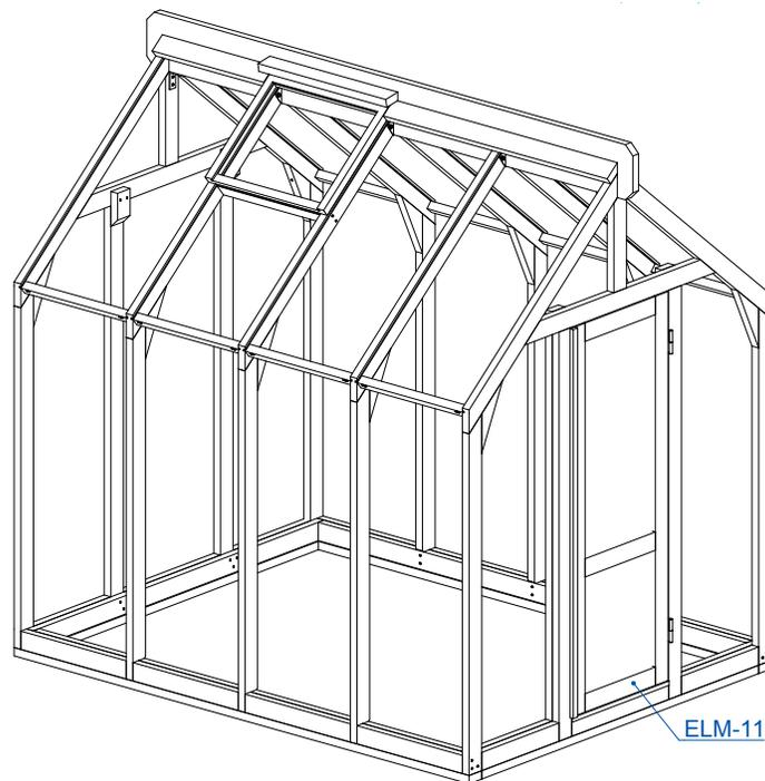
After the installation of the greenhouse and it is settled, then it may become necessary to adjust the height of the door. This can be done by adjusting the door hinges. Remove the hinge covers and turn the hinge adjustment screws until the door is in correct position.
