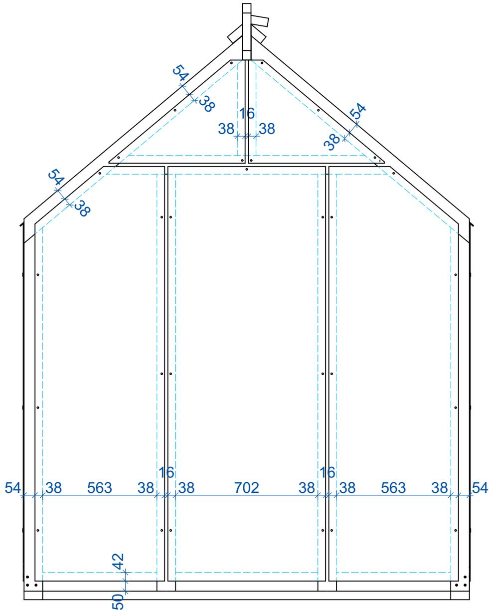
**NB! Make sure that the glasses are evenly spaced and that the attachment points line up. Observe the alignment of the glasses at their lower edge. The lower edge of the back wall glass must be 50 mm from base frame elements gap and line up with side glass lower edge.**
