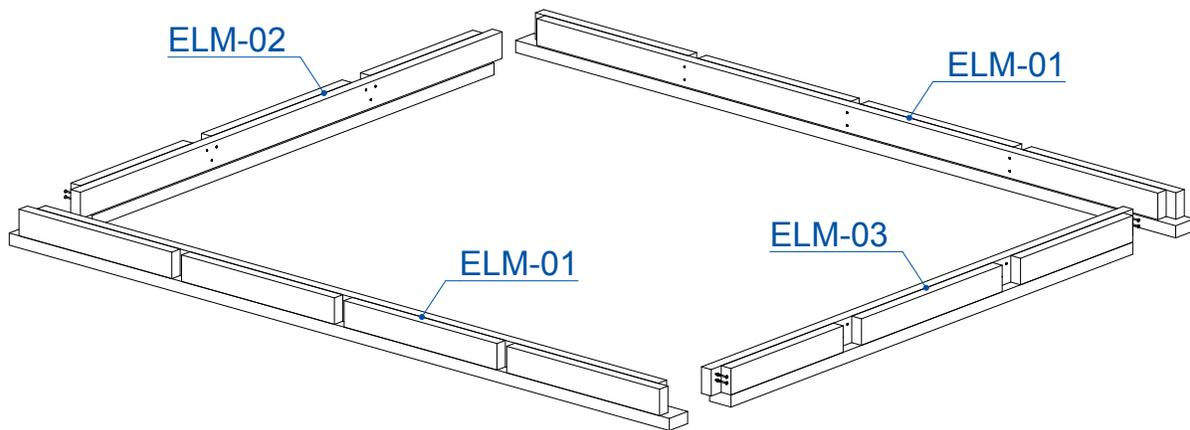
**NB! After installation of base frame, make sure that the corners of the greenhouse are 90 degrees and the diagonals are of equal length.**
