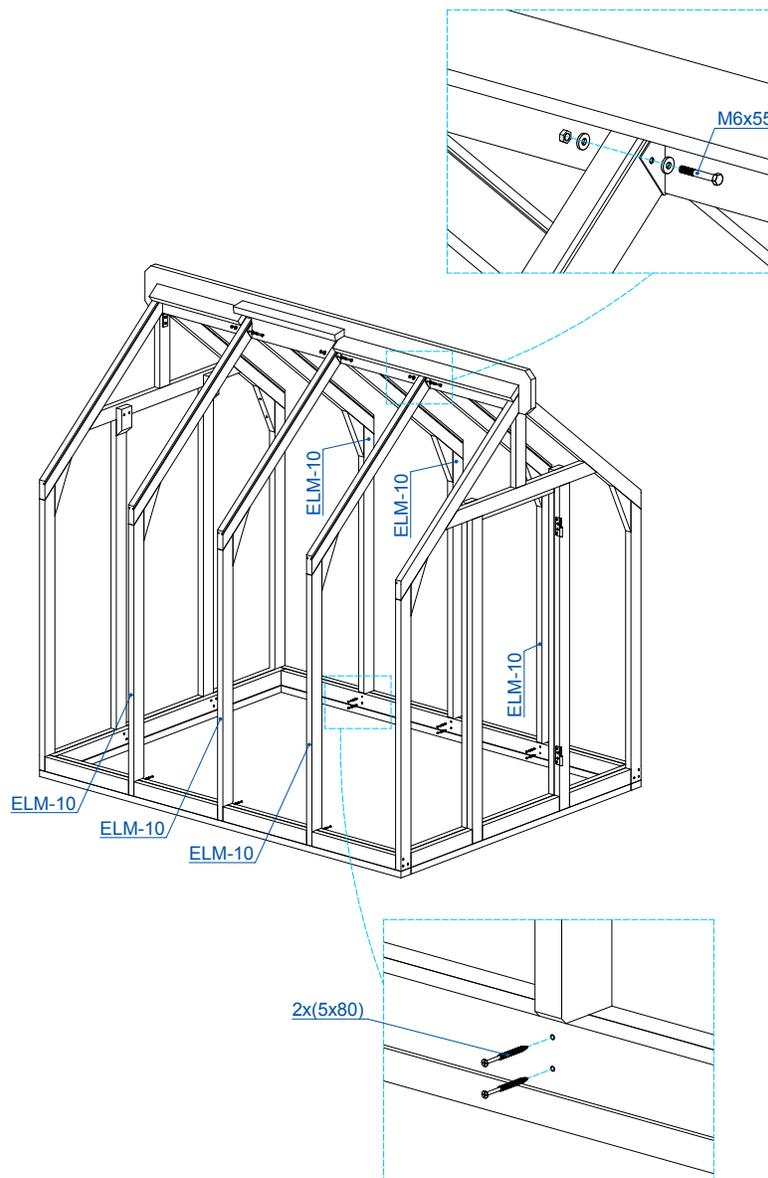
**NB! Tighten the nuts only later after installing the rafter middle details!
