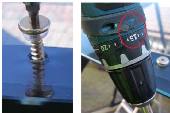
**The last part must be tightened ALWAYS by hand!!!**
