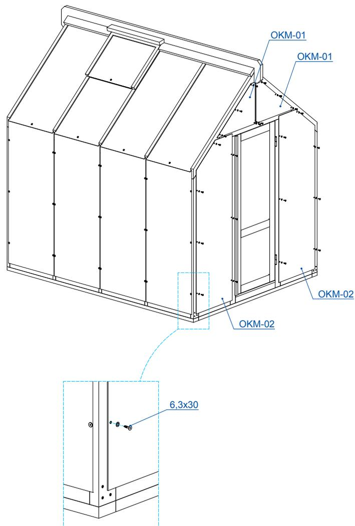
**NB! Make sure that the glasses are evenly spaced and that the attachment points line up. Observe the alignment of the glasses at their lower edge. The lower edge of the back wall glass must be 50 mm from base frame elements gap and line up with side glass lower edge.**
