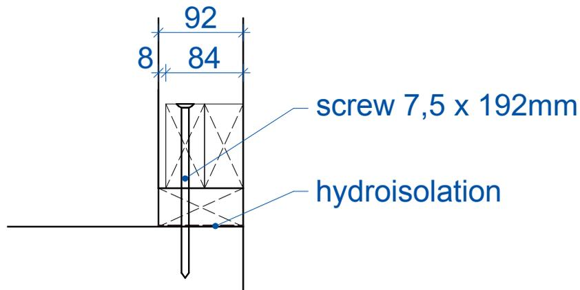
**NB! It is recommended to attach both ends and sides to the foundation.**
